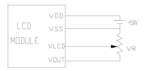
VDD-VLCD:LCD Drive Voltage VR:10K~20K
